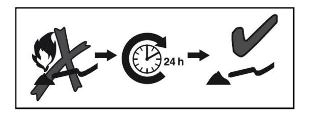
Wait at least 24 hours before vacuuming an oven or a fireplace in order to be sure that the fire has gone out and the ash has cooled down. Only for cold ash, see the operating instructions!
